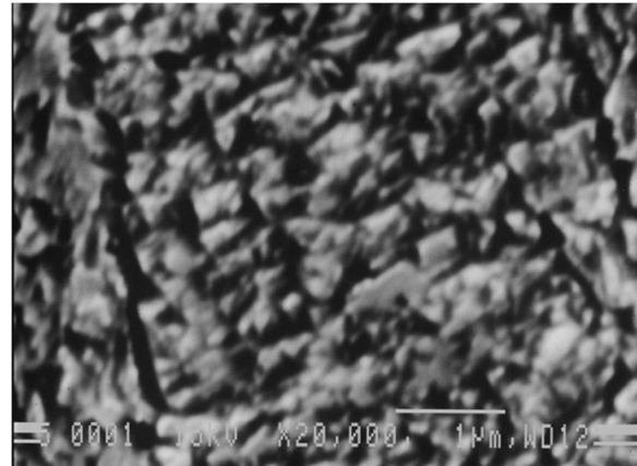
Fig. 18 SEM picture of the processed sample after single pass of PTCAE method.
