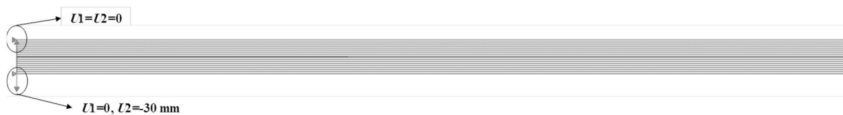
Fig. 6 DCB specimens boundary conditions
