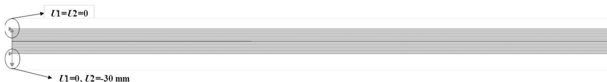
Fig. 6 DCB specimens boundary conditions
