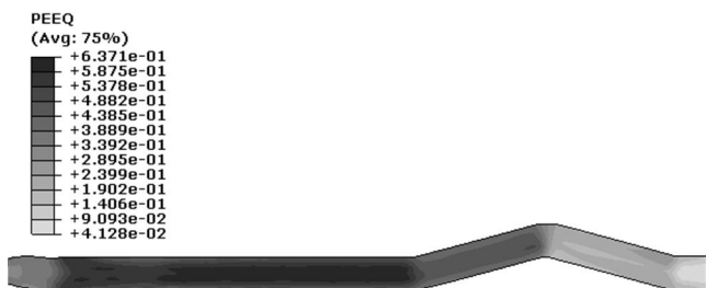
Fig 4 Deformed strips and equivalent plastic strain contour
