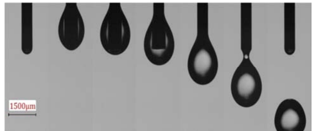
Fig. 2 Formation and separation of droplets in dripping mode, Flow rate= 6 ml/h, Voltage= 0.407kV
