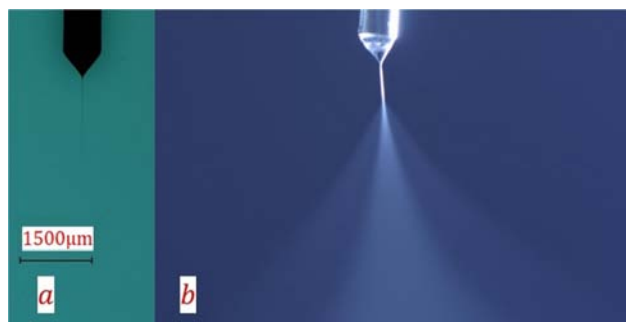
Fig. 13 Cone jet mode, (a): from shadowgraph, (b): from light scattering, Flowrate= 2 ml/h, Voltage= 4.63kV
