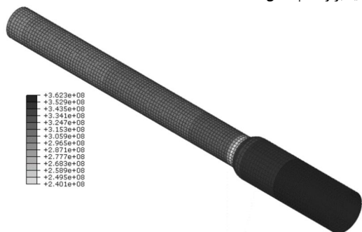
Fig. 21 Von Mises stress in composite vessel selected model caused by pressure load at the time of 7 milliseconds per pascal unit
