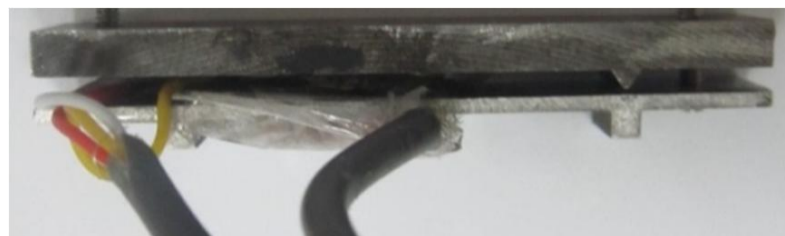
Fig. 4 strain gauge on aluminum pad
