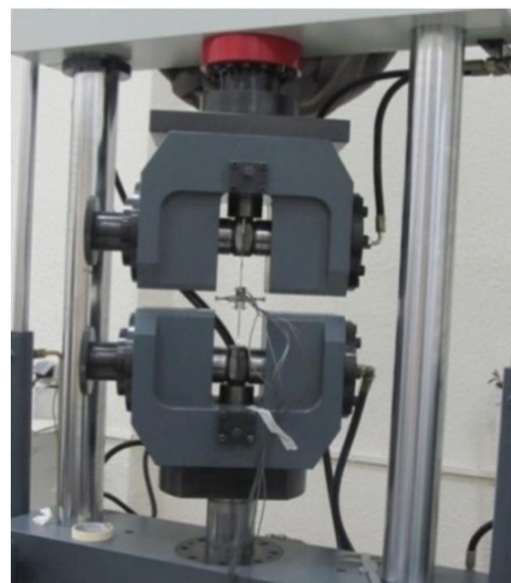
Fig. 5 fretting fatigue test assembly in fatigue machine
