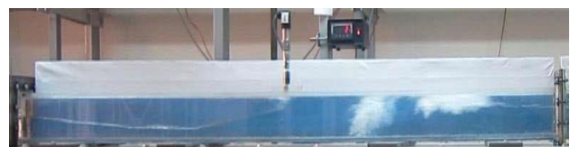
Fig. 2 Aerated slug flow in a duct [2]
