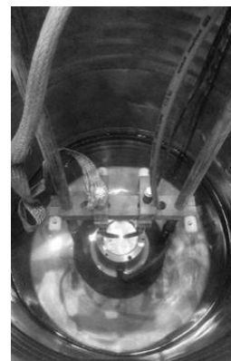
Fig. 4 Electrode system in the water chamber
