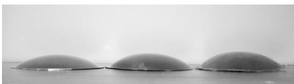
Fig. 10 Electrohydraulic deformed specimens
