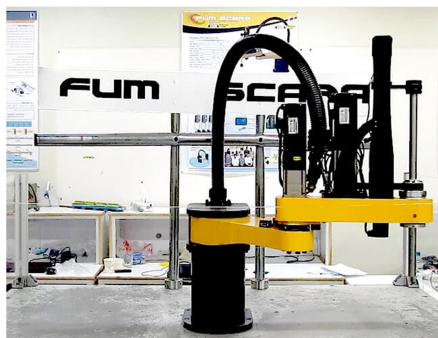
Fig. 3 The FUM SCARA robot designed and built at the Ferdowsi University of Mashhad, FUM Robotics Lab
