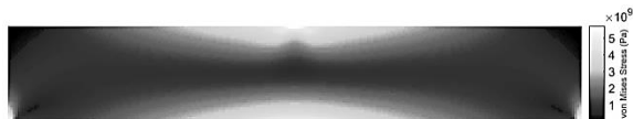
Fig. 7 von Mises stress plot in a structure with evenly distributed material equal to 30.72% of the initial domain
