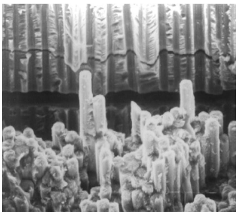
Figure 1 SEM photograph of fracture surfaces of a graphite/epoxy laminate [14]
