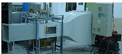
Fig. 2 view of open circuit wind tunnel
