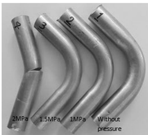
Fig. 11 Bent tubes in various pressures
