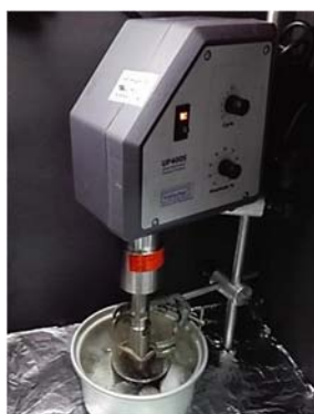
Fig. 2 Using of probe sonicator and ice bath
