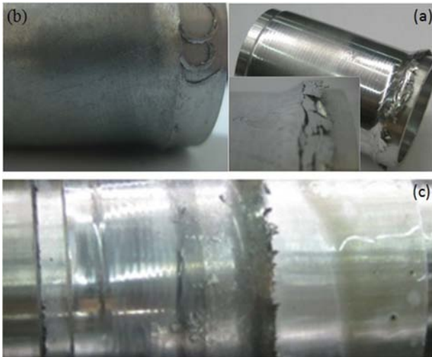
Fig. 3 Build-up of materials in front of rollers results in plastic instability and materials removing. Experiments conditions: feed rate 0.11 mm/rev, reduction (a) 33%, (b) 16.6% and (c) 33% to 16.6%
