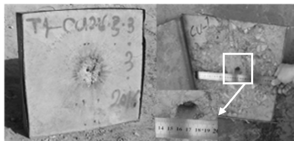
Fig. 8a First concrete target after forward projectile penetration (Right: back- Left: front)
