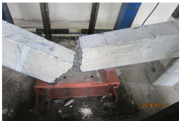
Fig. 12 Fracture of concrete under impact loading with drop hammer
