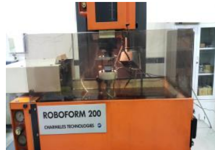
Fig. 4 The spark machine which was used at ultrasonic vibrations and magnetic field assisted EDM
