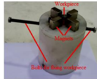
Fig. 3 The fixture which was used at magnetic field assisted EDM
