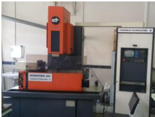
Fig. 1 The spark machine which was used for machining
