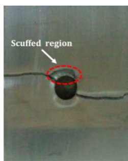
Fig. 10 scuffed region during cyclic loading
