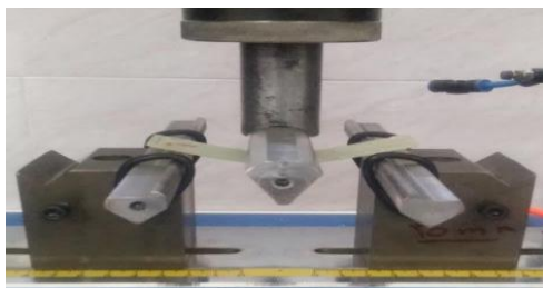
Fig. 3 Three-point bending test
