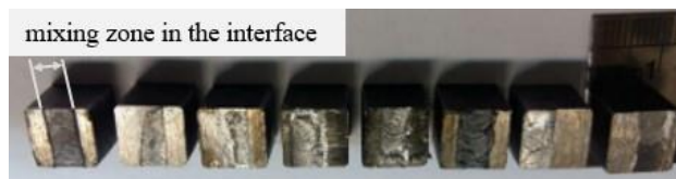
Fig. 12 Fracture surface samples tensile shear test
