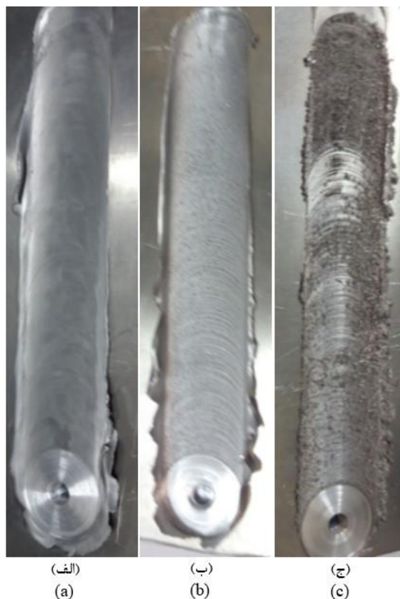
Fig. 11 The Surface flow of the cladding samples a) sample No.3 b) sample No.2 c) sample No.1
