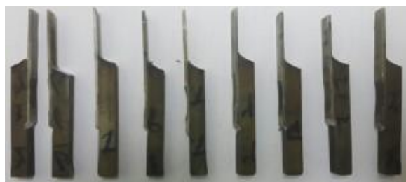
Fig. 6 Photograph of tensile shear test specimens
