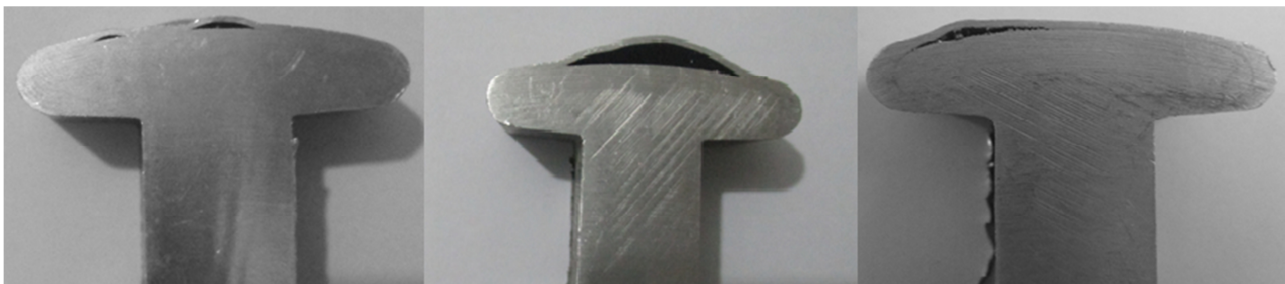
Fig. 12 The cracks created in crown part produced by using first die
