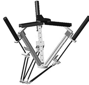
Fig.1 Schematic of a 3[P2(US)] parallel manipulator
