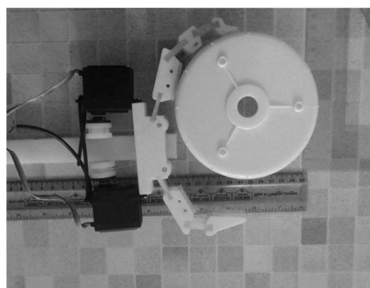
Fig. 12 The moved of gripper toward contact with object fixed on workspace
