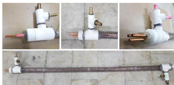
Fig. 3 View of the heat exchangers built with 1, 2, 3 inner tubes
