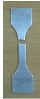
Fig. 12 A test sample after fatigue test
