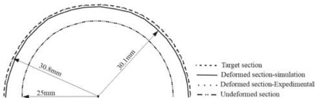
Fig. 11 Comparison of target profile with simulation and experimental profile for bulged sample
