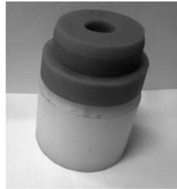
Fig. 7 Used Teflon and polyurethane for sealing
