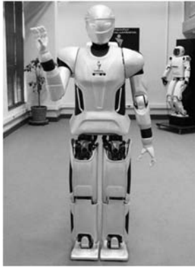
Fig. 1 SURENAIII humanoid robot
