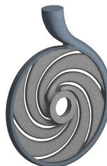
Fig. 3 Computational mesh for impeller and volute
