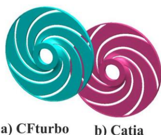
Fig. 1 Flow domain through impeller, a) CFturbo design b) Catia design
