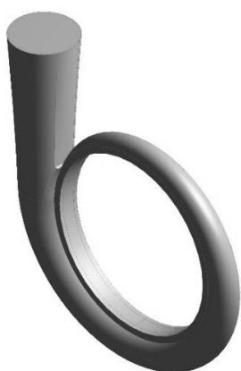
Fig. 2 Designed volute with CFTurbo software
