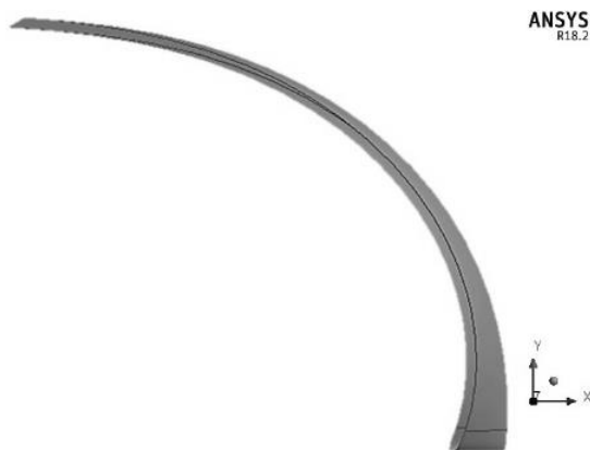
Fig. 16 The improve blade of centrifugal pump
