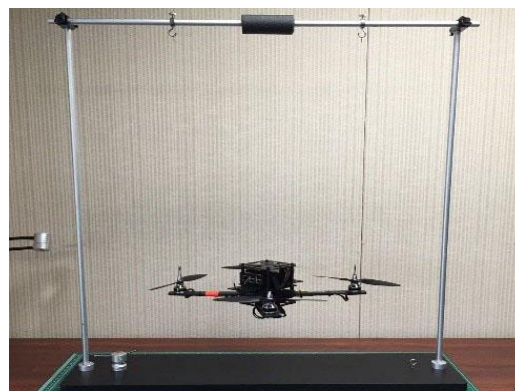
Fig. 3 Measuring moment of inertia by bifilar suspension method
