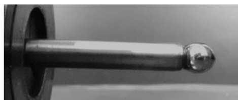
Fig.4 The hemispherical head tool with the 10 mm diameter
