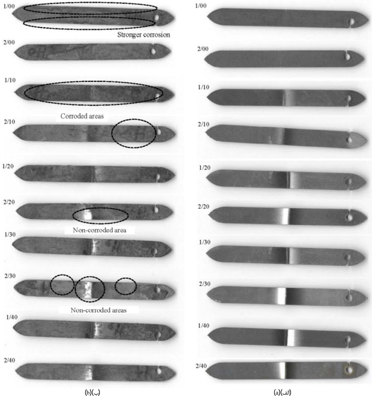
Fig. 8 Three layered sheet specimens; (a) before salt spray test, (b) after salt spray test
