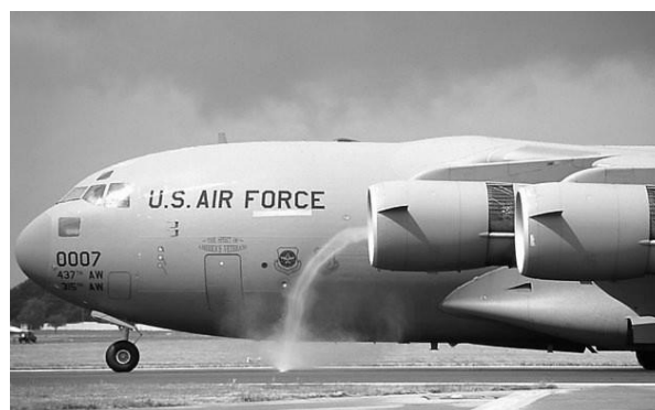
Fig. 1 Ground vortex on a military turboprop engine visible due to water condensation inside vortex core [4].
