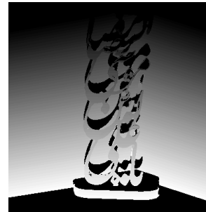
Fig. 14 Merging graycode series patterns
