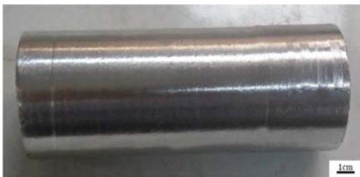
Fig. 3 Casting alloy sample after turning
